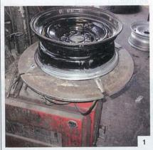
1 The old tires, with factory steel wheels, were dismounted from our test vehicle and the wheels inspected for any damage. The Hunter GSP-9700 will be used to measure both lateral and radial runout.
